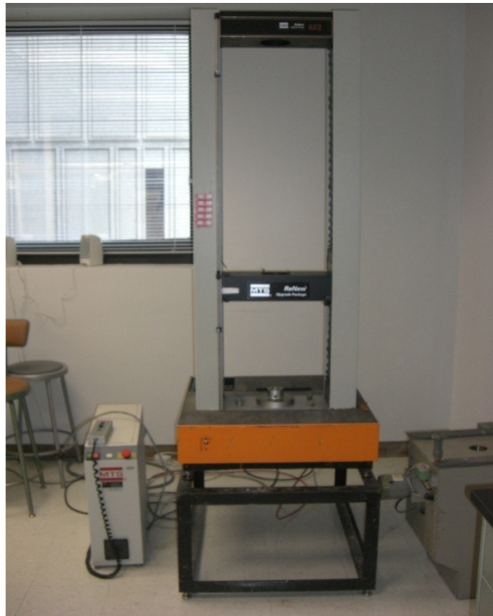
Figure 5: The MTS (Materials Testing System) Device used for force generation of Nitinol Implants
