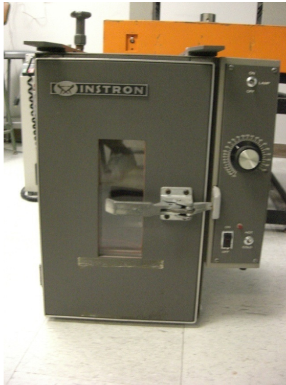
Figure 6: The Instron Environmental chamber used to observe changes in staples over a range of temperatures.
